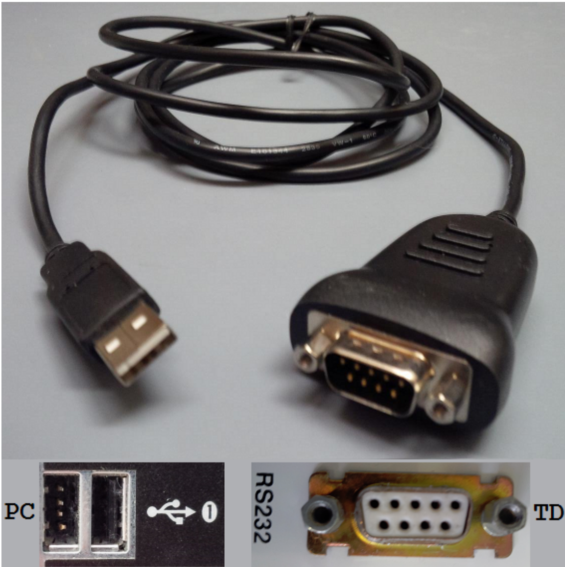
Figure 4.6: Optional serial-to-USB converter cable (top) can connect TD controller into USB port of PC and RS232 port of TD controller (bottom).
