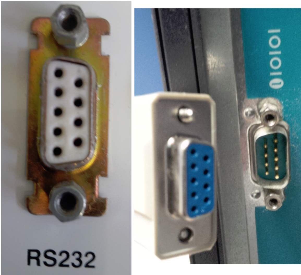
Figure 4.5: Serial ports on TD-5 (left) and PC (right). Connect serial cable (middle) between them. Your ports and cables may look slightly different.
