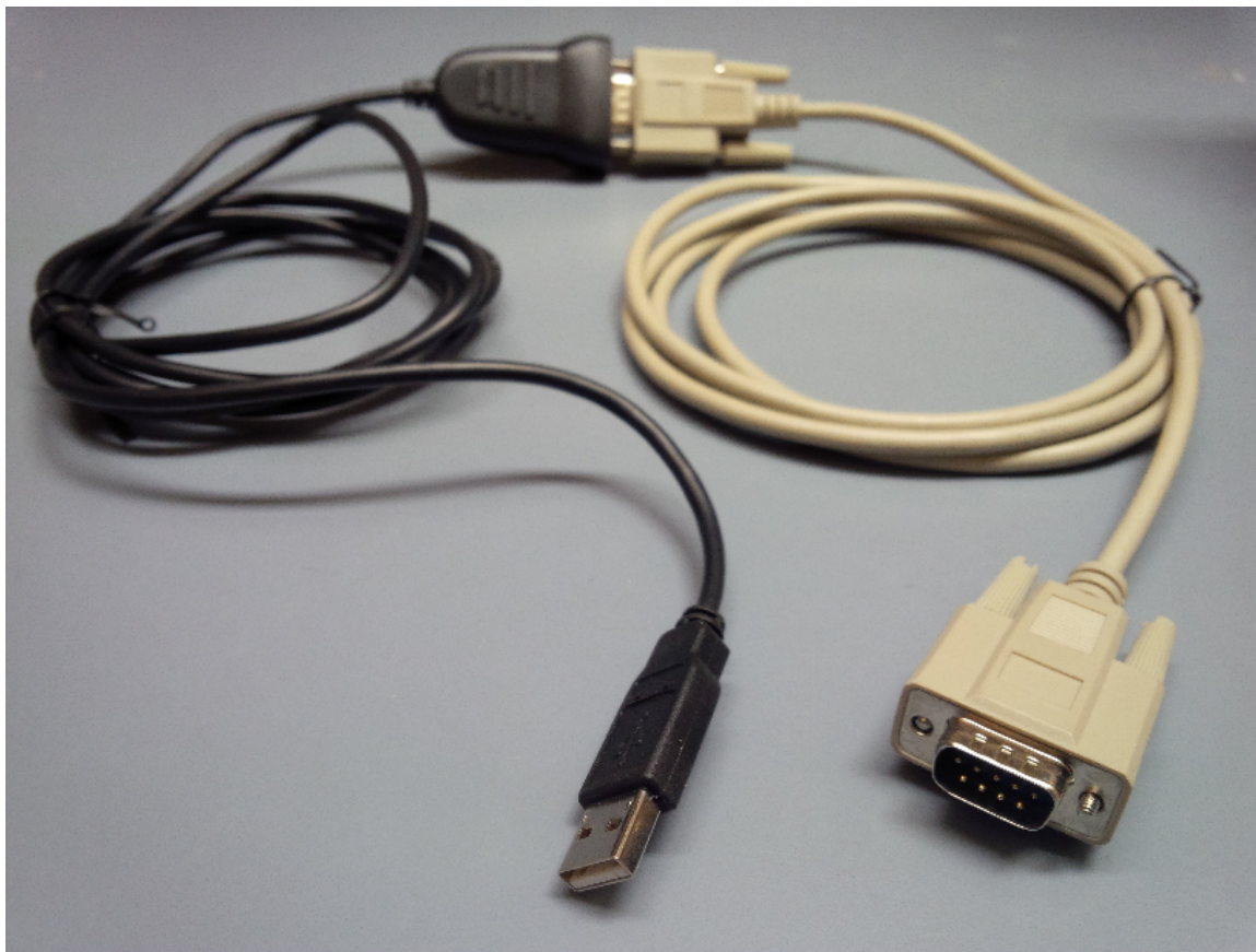
Figure 4.7: Optional serial-to-USB converter cable can be extended if needed with a serial serial cable.
