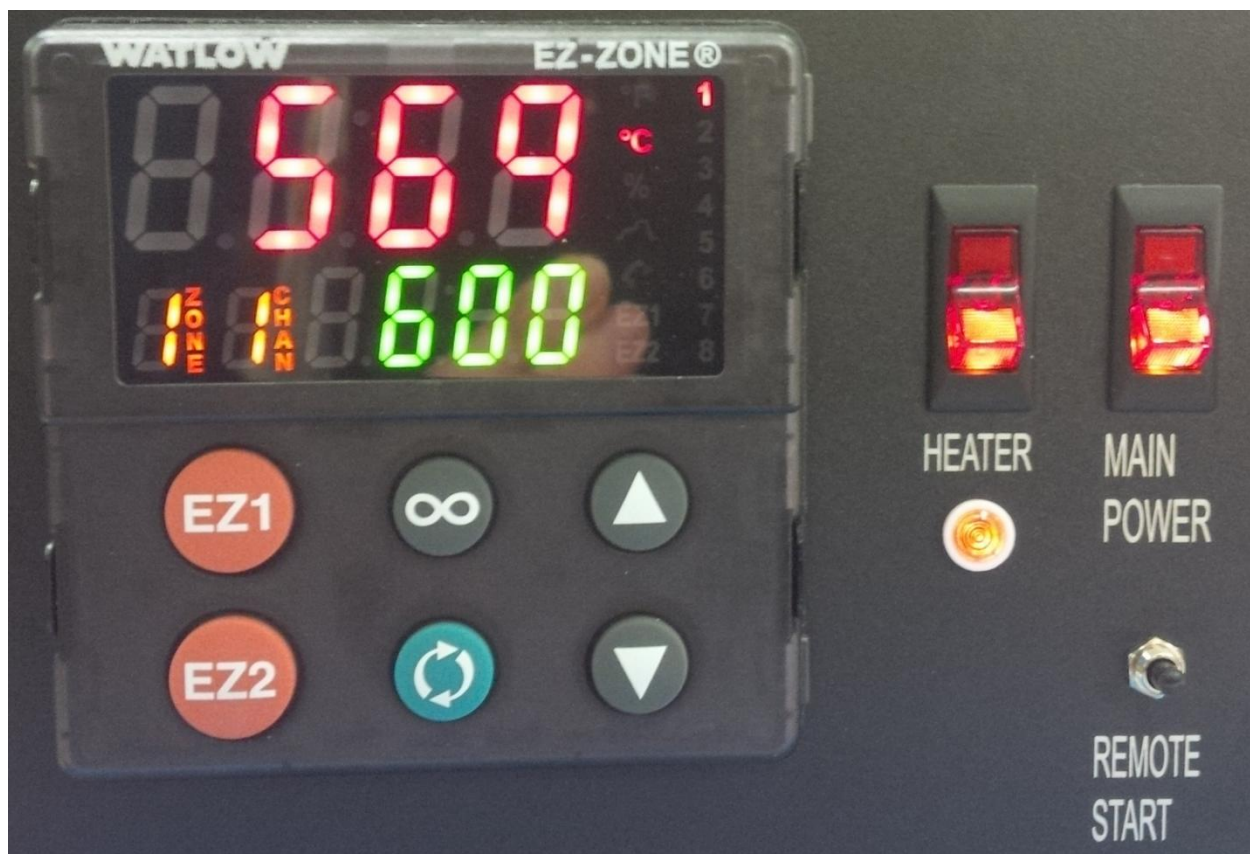
Figure 4: Temperature controller user interface (left) and other controls (right).
